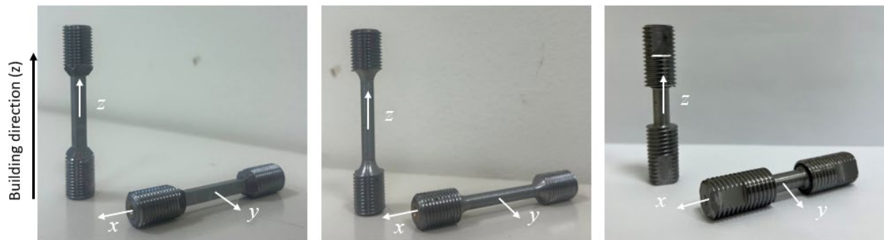
Figure 1 – Produced tensile (a) prismatic, (b) dog-bone and (c) torsion specimens: 0° (Z), 90° (X) orientation respect to z-direction
