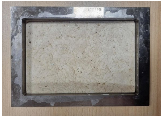
Figure 2 – 100 × 150 mm mould containing the composite material, prepared for the compression moulding process
