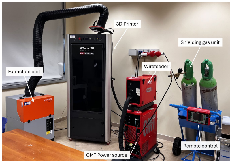
Figure 1 – WAAM-CMT set-up.
