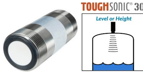
Fig. 4 ToughSonic 30 Sensor: Profile view and illustrative diagram of operation [10]
