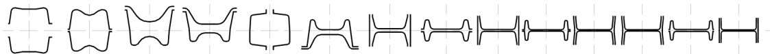
Fig. 3. The sequence of the passes in the mill “450” that is used for rolling the I-Beam IPE 160.
