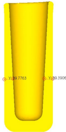
Fig .9. Double-process thermal extrusion forging bottom surface raised 250mm wall thickness map.
