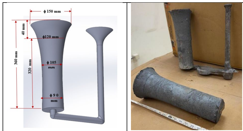
Fig. 4. presents schematic dimensional drawing and photo of the cast ingots.
