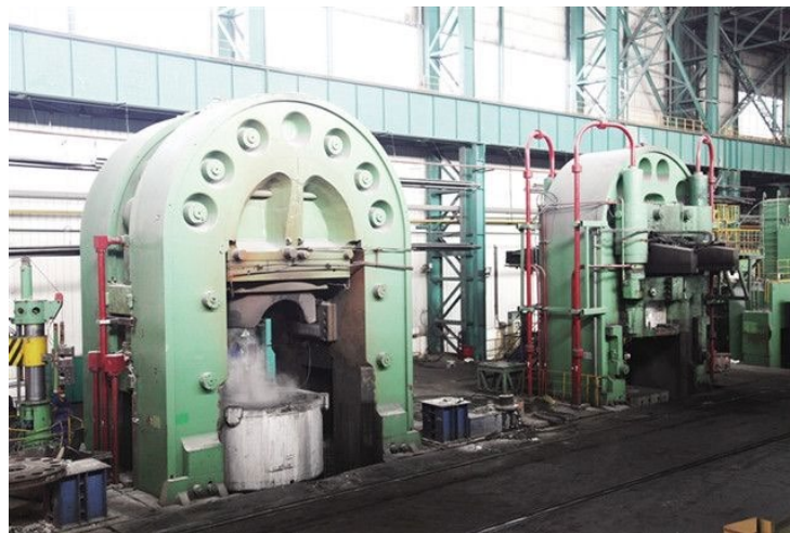
Fig. 1. 36,000 tons heavy vertical extrusion production line.
