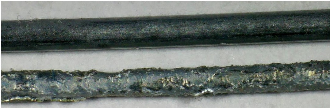
Fig. 3. Wire with an initial diameter of 1 mm before (top image) and after 28 days of corrosion (bottom image).
