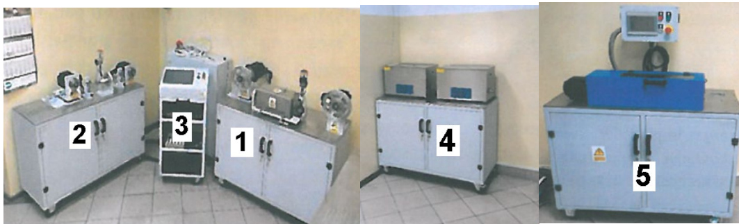
Fig. 1. Industrial technological line (INTERMECH Sp. z o.o.): 1 – the device for hot drawing; 2 – the device for cold drawing; 3 - the control electronic system; 4 – devices for ultrasonic cleaning; 5 - mechanical testing machine of the final wires.
