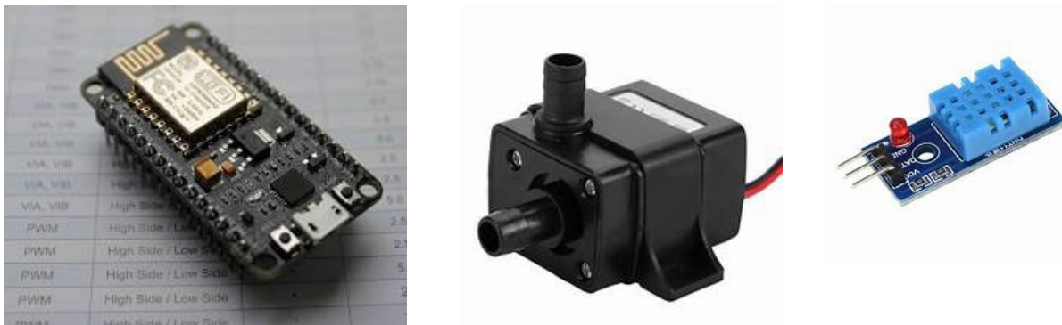
(a) (b) (c) Fig. 3 Components (a) NodeMCU, (b) Water Pump, and (c) DHT11
