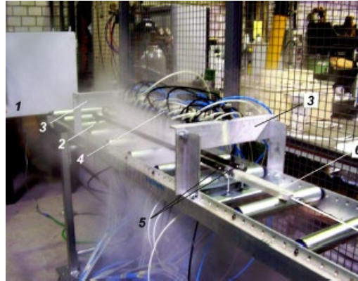
Fig. 1. Water-air cooling installation: 1 – furnace; 2 – roller conveyor; 3 – frame; 4 - holder with nozzles; 5 – guides; 6 - sample with installed thermocouples [8]
