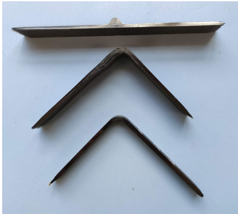
Figure 5. The three stages of manufacture outlined in this paper. Top is the initial MMCRC 'flat' panel, with a vitrimer excess length region and typical epoxy arms. The middle is the panel after forming, with ply separation present due to vitrimer flow. The bottom section is the final panel after consolidation.
