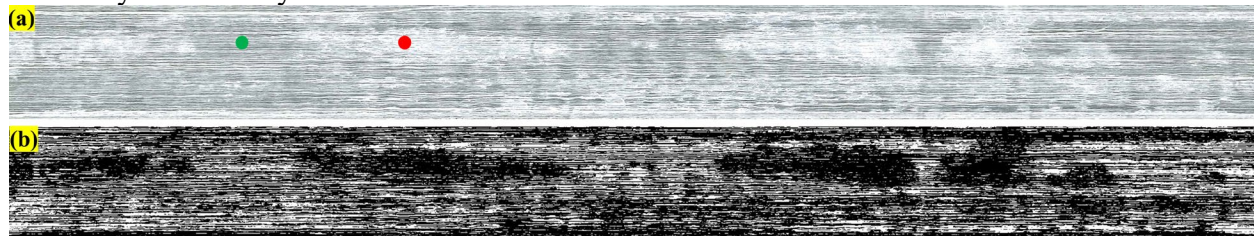
Fig. 10. (a) an image of the delaminated surface and (b) its thresholding result of a S4 sample
