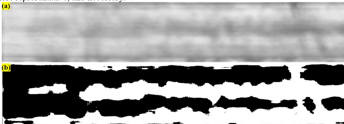
Fig. 9. (a) the C-scan image and (b) its thresholding result of a S4 sample
