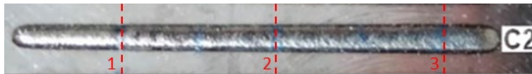
Fig. 5: Graded bead deposited at V_s = 0.9 [m/min], F = 25 [g/min] and P = 1450 to 2550 [W].
