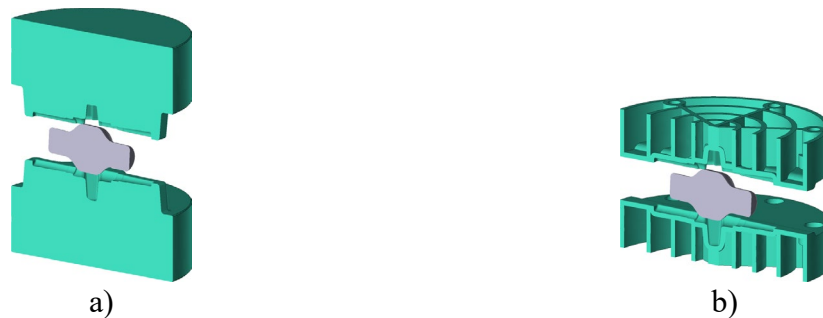
Fig. 6. The section cuts of the geometry models used in the forging simulation with WA-DED (a) and L-PBF (b) die
