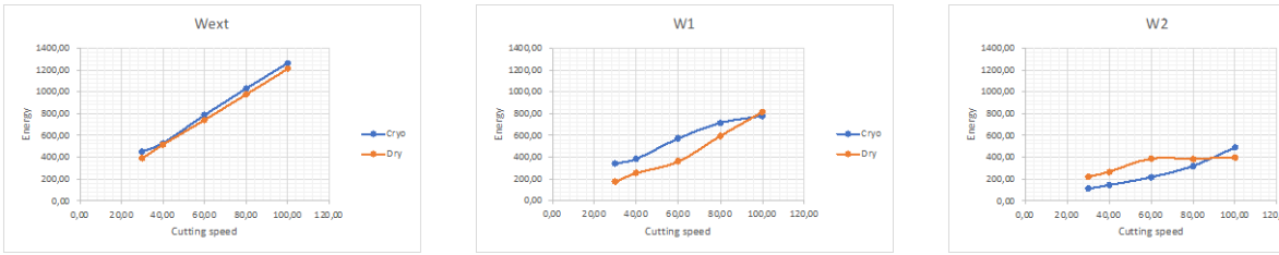
Figure 5 : Evolution of energies when cutting speed increase
