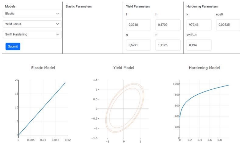
Fig. 7. Example of behavior model representation in the VForm-xSteels Front end. The model is composed of an elastic law, yield criterion and hardening law.
