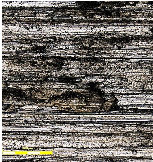
Fig. 7. Surface morphology after sliding contact under technically dry friction.
