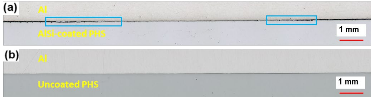
Fig. 6 Typical cross-sectional macrostructures of the joining interface in the stirred zone (SZ) of samples (a) with and (b) without the AlSi coating layer (RotSpeed: 2400 rpm, PluSpeed: 1 mm/s, DweTime 0 s, PluDepth 1.1 mm).
