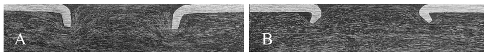
Figure. 5 Cut section of specimens A) Specimen without edge interlock. B) Specimen with edge interlock.
