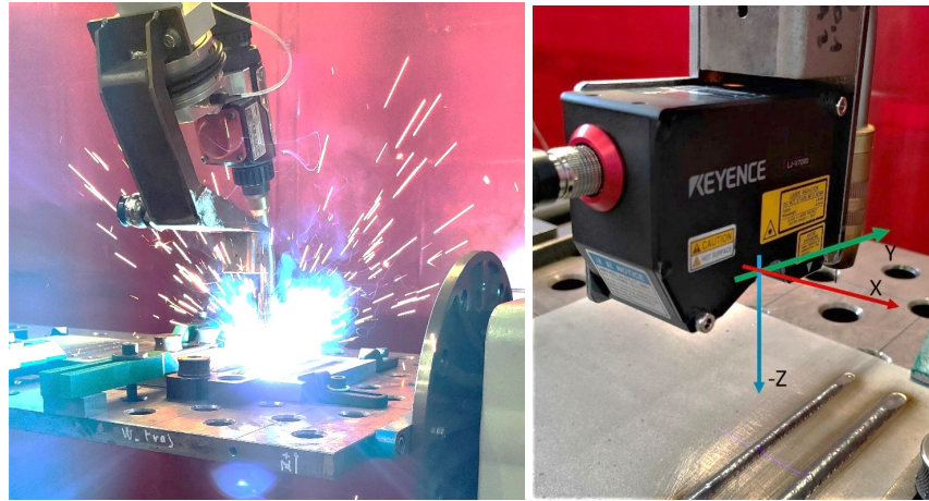
Figure 1: (a) WAAM-CMT Process (Laser tracker reflector visible on the left side) (b) Laser scanner used for the capturing the bead profile
