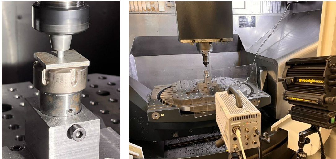
Fig. 2. Photos of experimental set up (on the left with a high-speed camera and the dynamometer, and in the right the tool just before touching the rivet – the square protection plate is not attached to the rivet nor the cone)
