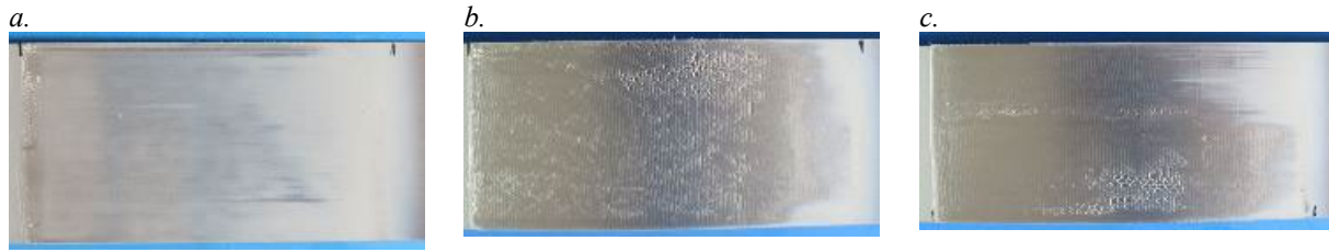
Fig. 5. Photograph of samples for tool temperature of 195 °C with normal force of a. 2kN, b. 4 kN and c. 8 kN. Tool side with large radius. Drawing distance from right to left.
