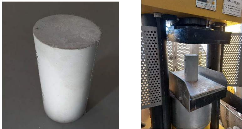
Fig. 1. Concrete specimens prepared for compressive strength test.
