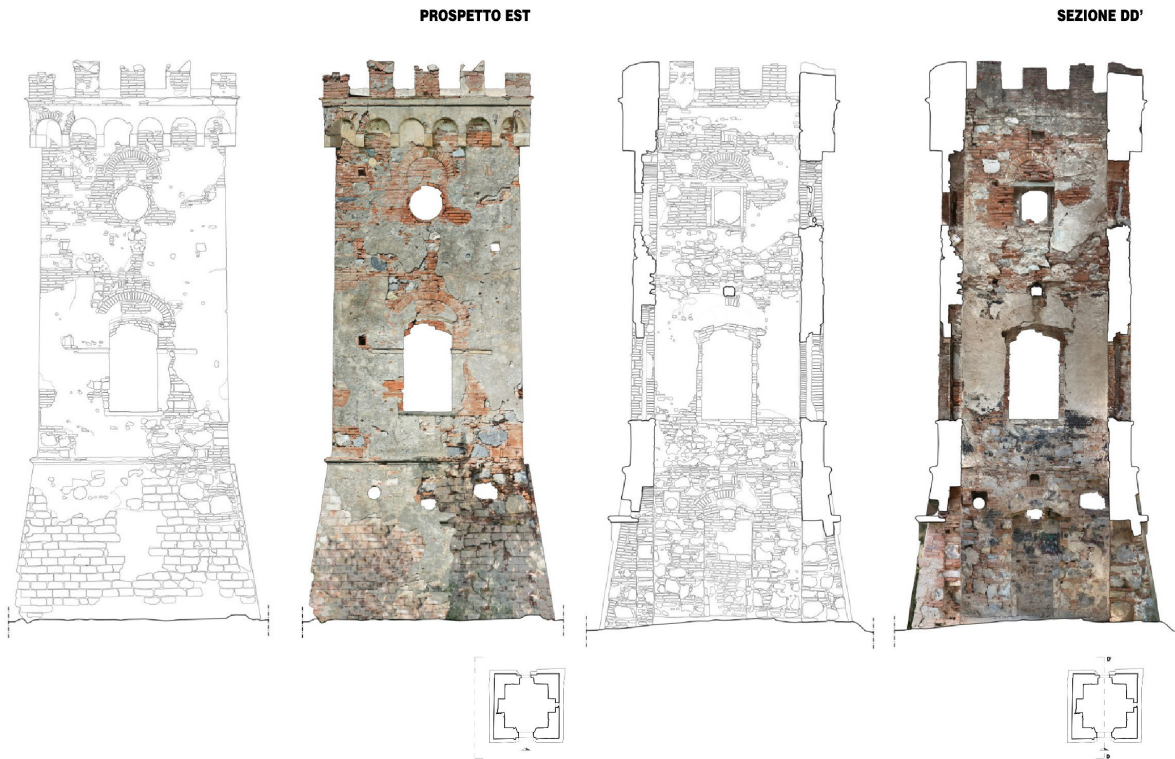
Fig. 9, The East elevation, on the right, and the elevation section D-D', were first rendered with the wireframe, and then with the photomap on the right.
