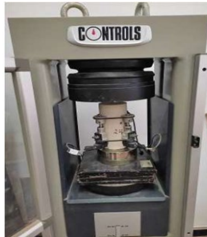
Figure 8: Picture of the compression machine taken in the NSAS laboratory
