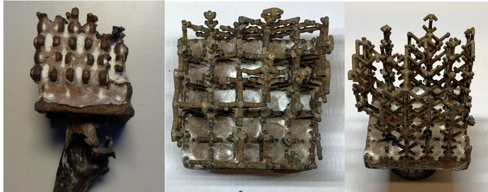
Fig. 2: Results of the first trials for casting structures with high manganese steel
