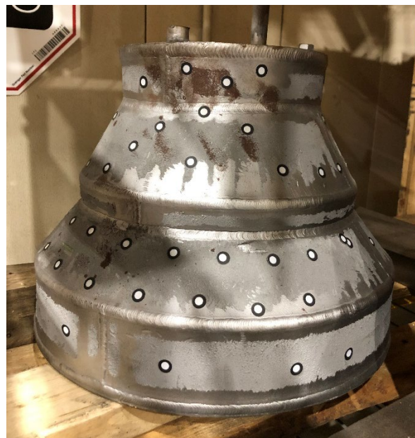
Figure 6. Experimental capsule post-HIP (dots for 3D scanning)
