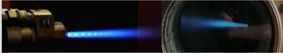
Figure 8 – HVOF gun at ambient pressure (left) and in the VOF Test Chamber (right).
