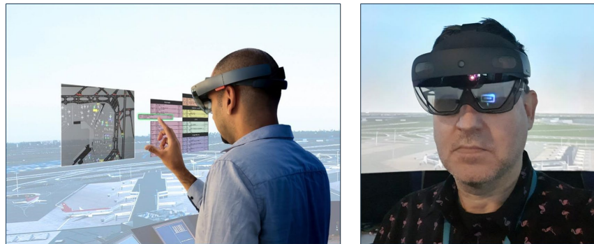
Fig. 2: Innovative Use of AR Devices in the Aerodrome Tower (e.g. EFS, Adaptive Labelling )
