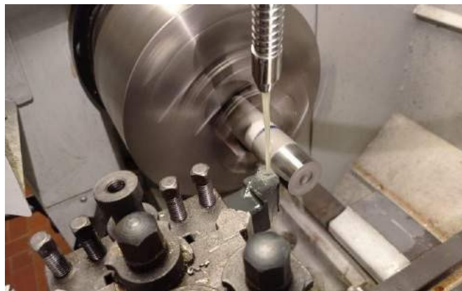
Figure 1. Post-process turning of the EBM Ti6Al4V sample with the lubricant
