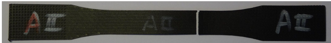
Fig. 6. Test specimen No 2 of the sample set A after the static tensile test.
