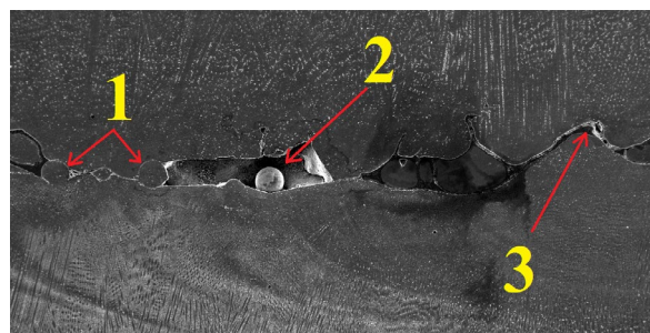
Fig. 3. Discontinuities in material manufactured using the powder deposition method.
