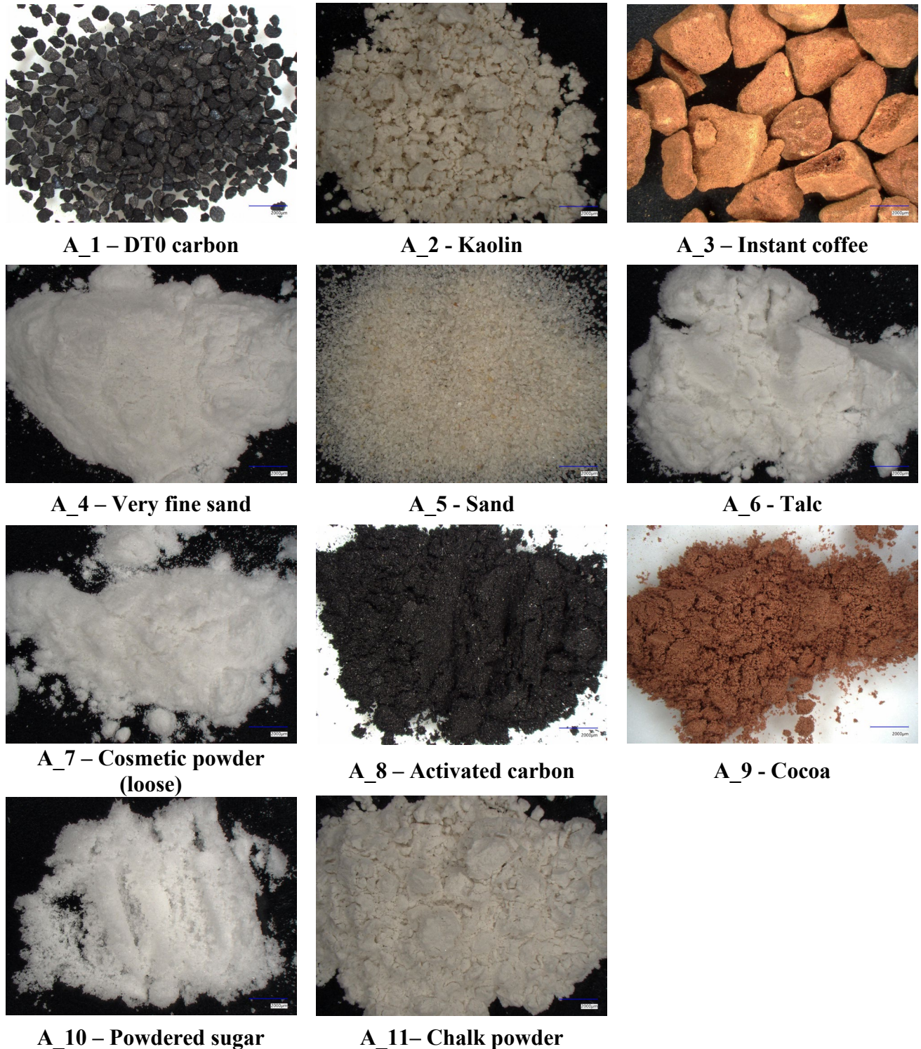
Fig. 3. Optical microscope photographs of powdered and loose materials serving as admixtures in the created two-component mixtures with AN
