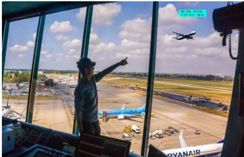
Figure 1: Retina Concept: an ATCO with the ST-HMD visualises the Aircraft Tracking Label through the window of the Control Tower.
