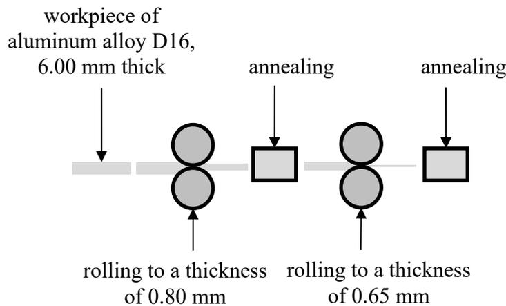
Fig. 2 – Process flow chart of asymmetric rolling of the narrow strip from aluminum alloy D16 with work roll speed ratio  $V_1/V_2 = 10.0/2.0$
