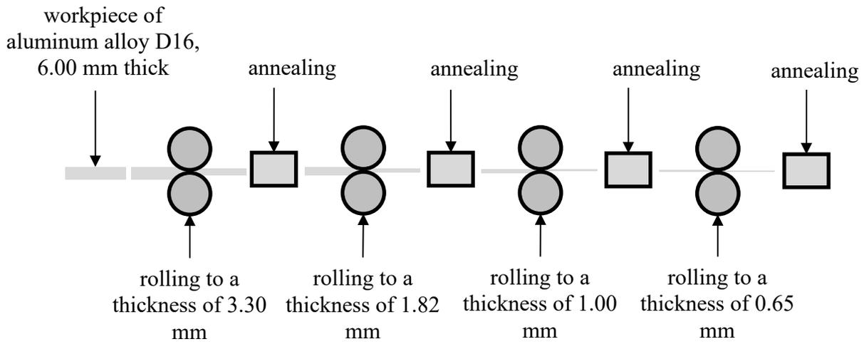
Fig. 1 – Process flow chart of symmetric rolling of the narrow strip from aluminum alloy D16
