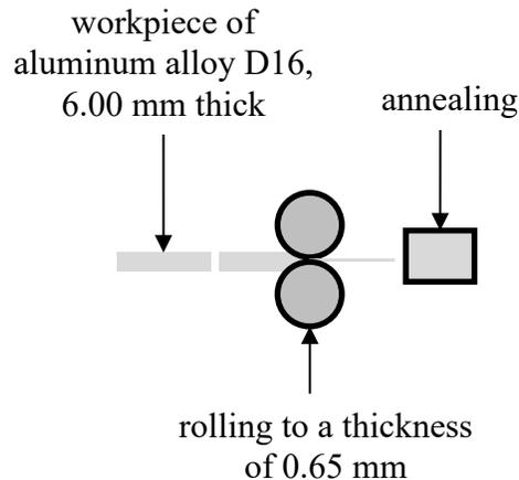
*Fig. 3 – Process flow chart of asymmetric rolling of the narrow strip from aluminum alloy D16 with work roll speed ratio  $V_1/V_2 = 10.0/1.5$*
