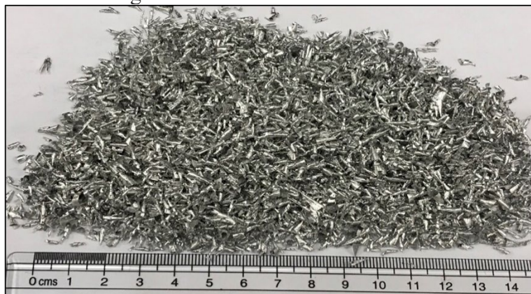
Figure 1 AZ31 Mg alloy chips generated by milling machine.
