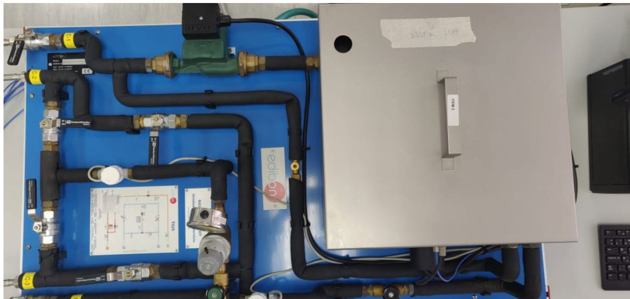
Figure 1. Base unit includes: hot fluid tank, sensors, valves, pump and pressure regulator
