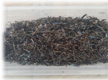
Figure 4: Machining metal fibers (length 13 mm, diameter 160 μm)
