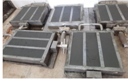
Figure 6: Casting of specimens
