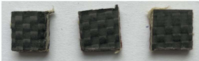
Figure 2. C-B-A reinforced hybrid composite specimens from left to right, respectively; no aging process was applied, 12 h aging process was applied and 48 h aging process was applied.
