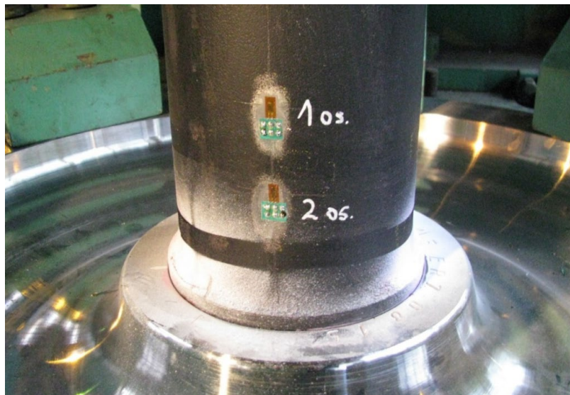
Fig. 1 View of the arrangement of resistance strain gauges
