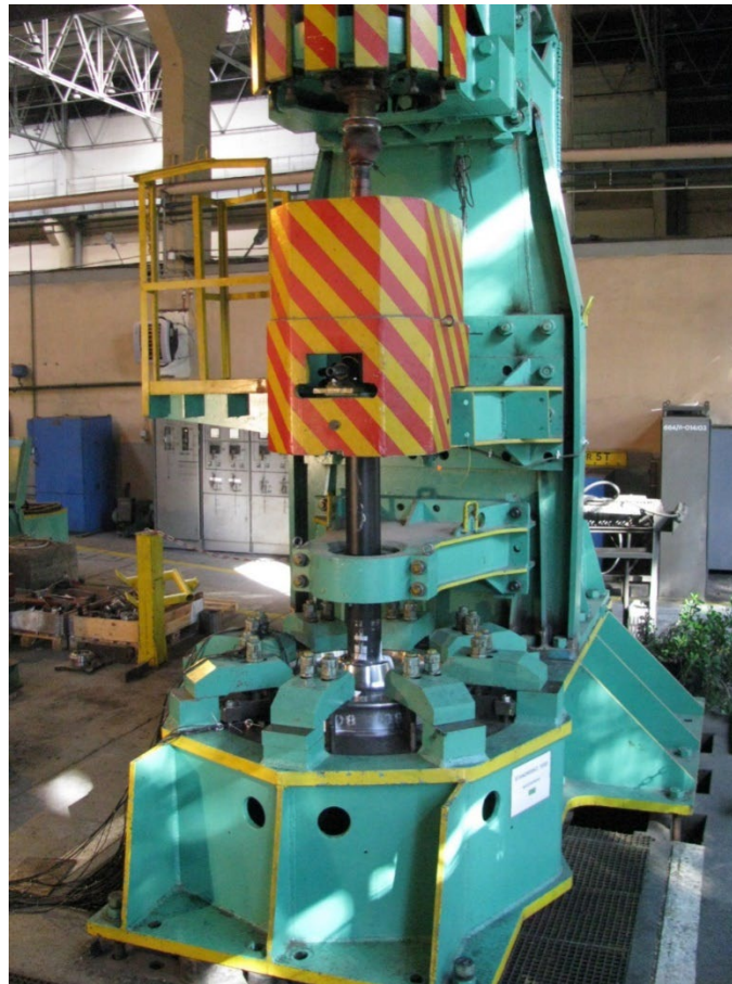
Fig. 3 View of the fatigue machine for testing axles and wheels of wheelsets (Łukasiewicz-PIT archive)
