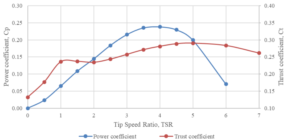
Fig.9 Power and thrust coefficient performance of the turbine against TSR.
