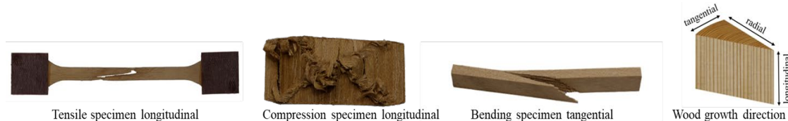
Fig. 2. Black locust test specimen for mechanical characterization.
