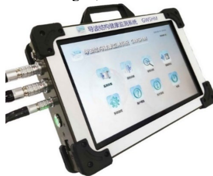
Fig.3 compact and portable piezoelectric guided wave structure health monitoring system
