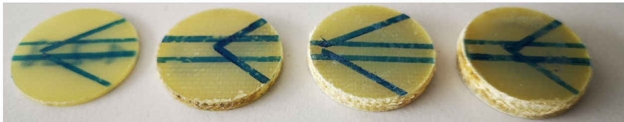
Fig. 3: Cut slugs featuring thicknesses of 1, 2, 3 and 4 mm from left to right
