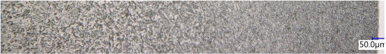
Fig. 5. Microstructure of reinforcing steel in the axis of the specimen. The white region is an unetched martensite steel side.
