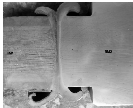
Fig. 4. Macrostructure of the joint with asymmetrical flashes
