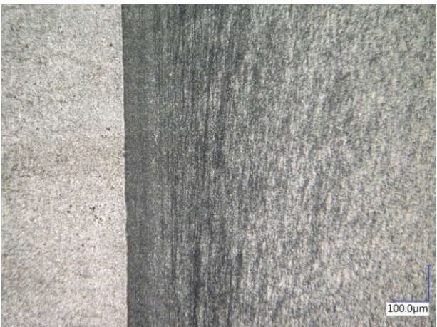
Fig. 7. Thermo-mechanically affected zone (TMAZ) in the 1.4021 steel (on the right from weld)
