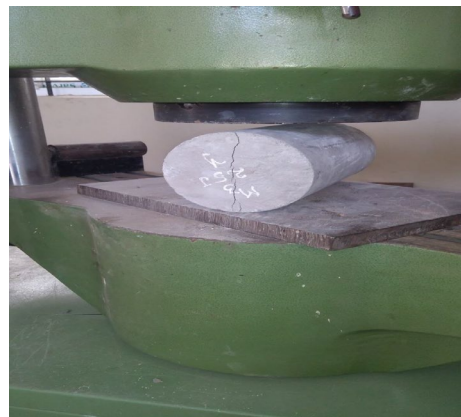
Fig.6 - split tensile strength test
