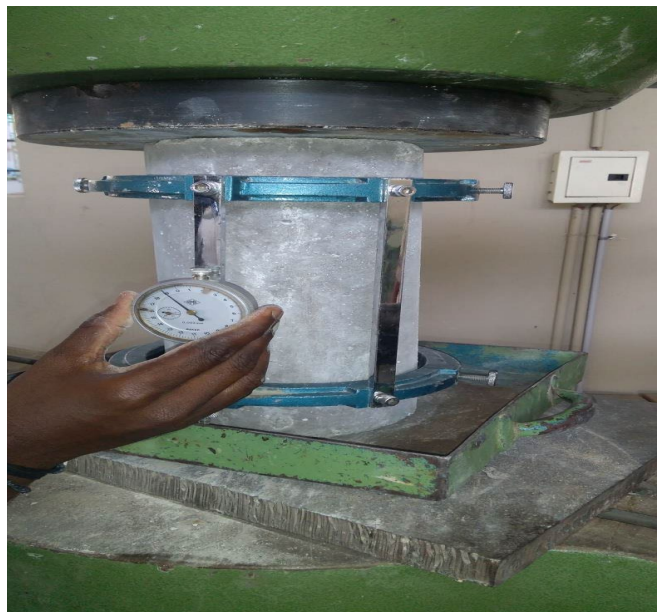
Fig.8 – Modulus of elasticity test set up
