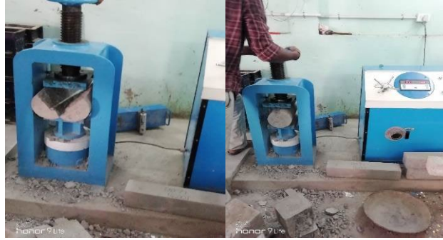
Fig 4: Split tensile on GF Concrete
