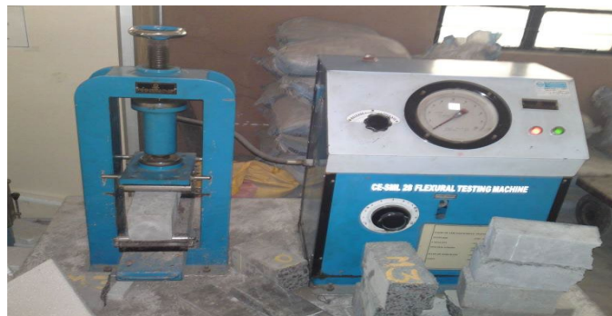
Fig 5: Flexural strength test
