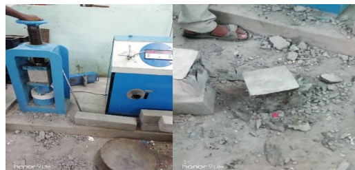
Fig 3: Compressive strength on GF Concrete
