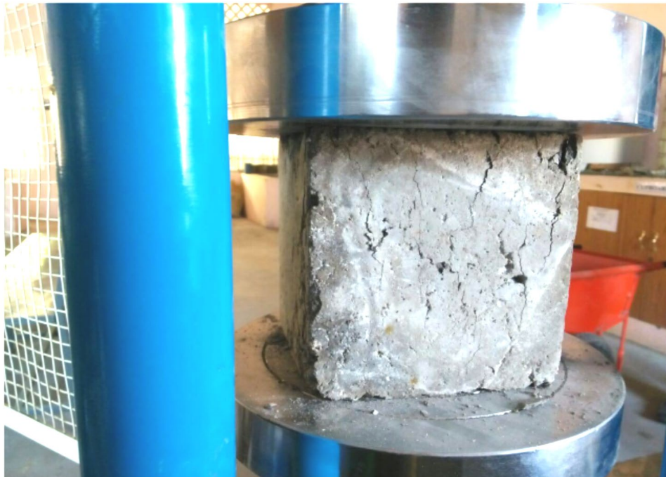
Fig. 2: Compressive Test of Concrete Cube
