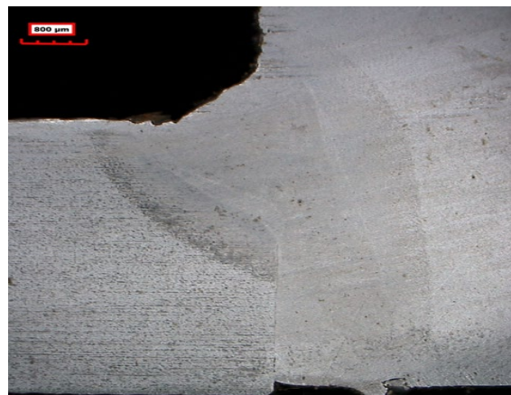
Fig. 6. Macrostructures of partial lap joint weld in cross section.
